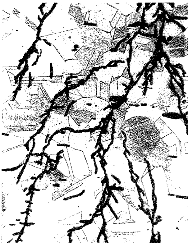
Figure 21. Photomicrograph at 400x magnification showing typical transgranular, branched, cracking of 304 stainless steel in a hot chloride environment.
