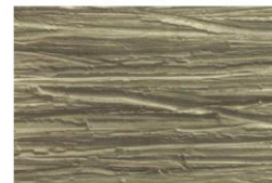
Figuur 2.16.6: Abrasieve slijtage (high stress)
